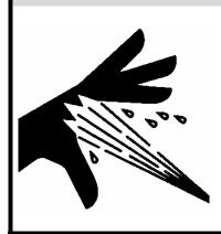
Component failure may result in high-temperature oil spray, causing serious injury or death.
